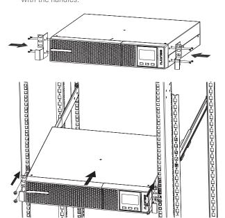
Fig. 5. Rack-type mounting in a 19" cabinet.
