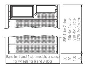
Height of the different sub-racks according to the number of slots
