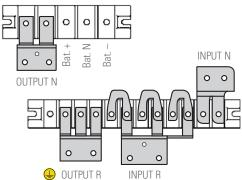
Terminal block in 2-slot and 4-slot sub-rack.
