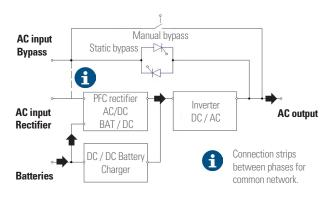
Fig. 19. Flowchart in Battery Mode.
