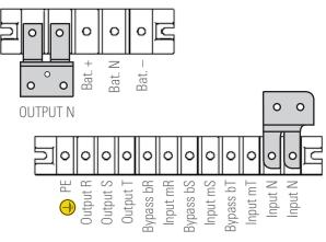
Terminal block in 2-slot and 4-slot sub-rack.
