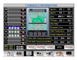
Fig. 57. Information menu of the module or power modules. Information sub-menu.
