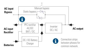
Fig. 18. Flowchart in Normal Mode.
