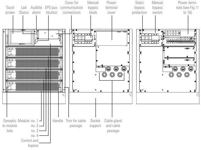
When installing a sub-rack inside a cabinet, the static bypass and manual bypass switches on the back of the sub-rack will be inaccessible. In relation to the first one, it is necessary to set it to "On" before placing the sub-rack in the cabinet. The figure on the right shows the sub-rack with the terminal cover removed.
