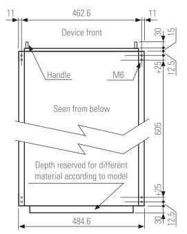
Dimensions for fixing 2 and 4-slot sub-racks through their bases
