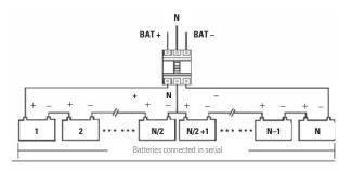
*Fig. 32.* Typical connection of battery set.
