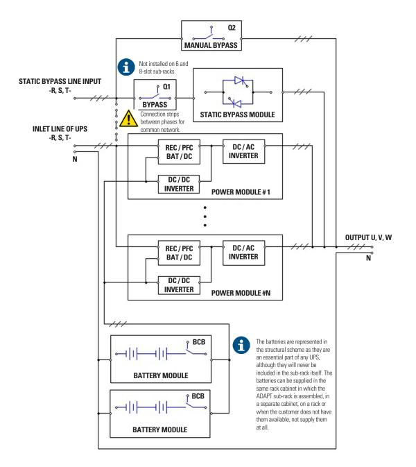
Fig. 10. Single-line structural diagram by way of example.
