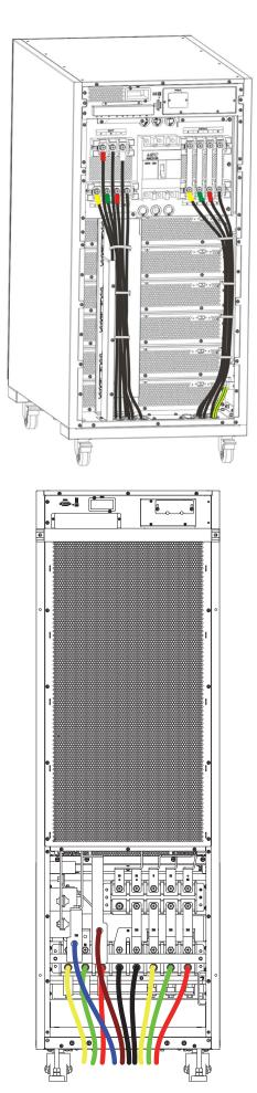
Fig. 31. Cable entry on 6 and 8-slot sub-racks.
