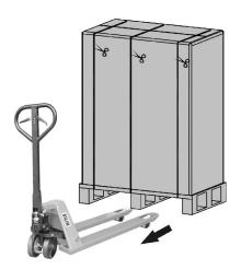
Fig. 24. Example of transfer of packed ADAPT X with pallet jack.
