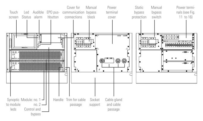
When installing a sub-rack inside a cabinet, the static bypass and manual bypass switches on the back of the sub-rack will be inaccessible. In relation to the first one, it is necessary to set it to "On" before placing the sub-rack in the cabinet. The figure on the right shows the sub-rack with the terminal cover removed.
