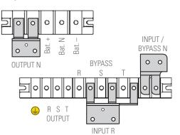
Terminal block in 2-slot and 4-slot sub-rack.
