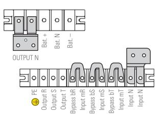
Terminal block in 2-slot and 4-slot sub-rack.
