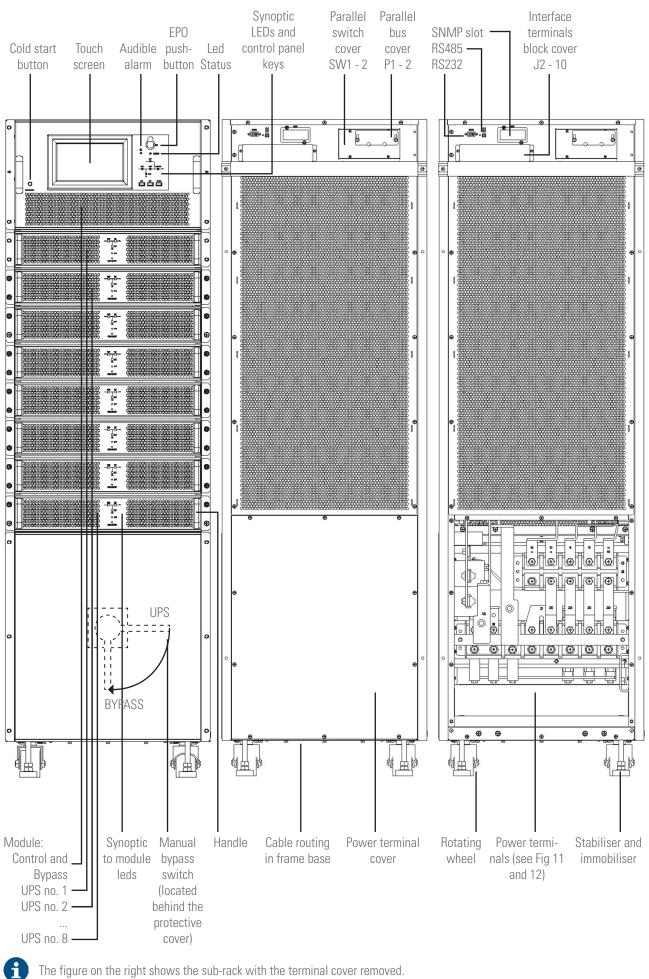
Fig. 4. Sub-rack model with 8 slots.
