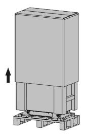
Fig. 25. Example of removal of cardboard box.
