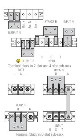
*Fig. 15. Three-phase/single-phase configuration and separate networks.*
