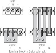
Fig. 13. Single-phase/single-phase configuration and common network.
