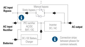
Fig. 20. Flowchart in Bypass mode.
