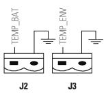
*Fig. 66.* Terminal block J2 and J3 for connection with sensors.
