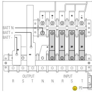
Terminal block in 8-slot sub-rack.
