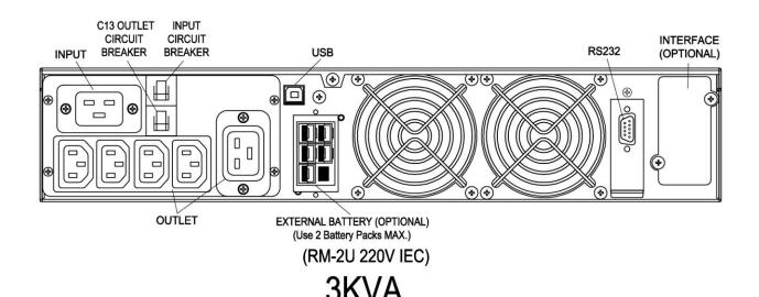
Rear panel of UPS 1KVA to 3KVA (Rack Type)
