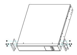
Attach two rack mounting ears to UPS, using provided M5 screws 8pcs.
