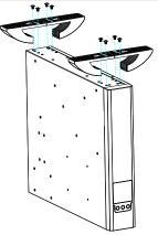
Attach four rack tower stands to UPS, using provided M5 screws 8pcs.
