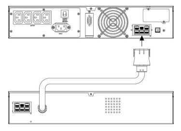
Example of connecting to external battery pack
