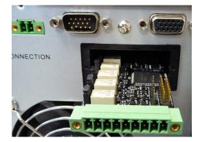
Fig. 8. Inserting the NIMBUS AS400 card
